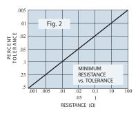
How You Can Profit From PLV Shunts: Variable lead sizes ...... for current-sensing to 45 Amps Resistance values ...... to  $0.001\Omega$ Voltage drop or ohmic tolerances ...... to  $\pm 0.005\%$ TCR characteristics ......15ppm/°C (std.) to 10 ppm/°C Temperature Span ......-65 to +275°C @ 1% tolerance For closer tolerance see Derating Curve Fig. 3
